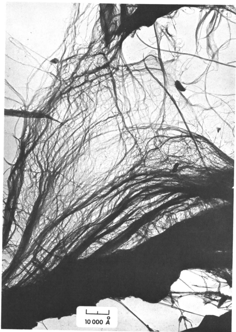
Figure 6. Transmission electron micrograph of the trimethylsilyl polymer showing the flexibility of its fibers.
